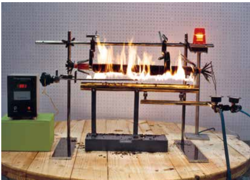
3 Hours fire survival test as per IEC-331
